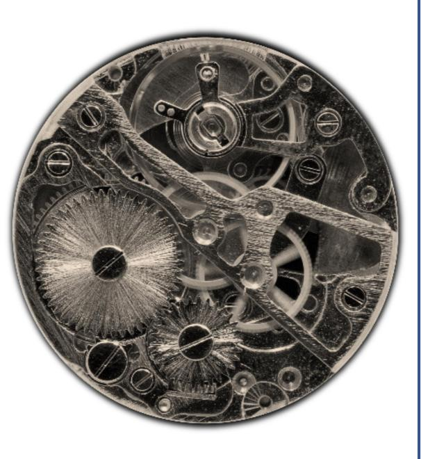
AT THE CENTER OF THE BALANCE WHEEL AND OTHER FRICTION POINTS ARE THE WATCH'S 'JEWELS,' ORIGINALLY RUBIES OR SAPPHIRES (REPLACED BY SYNTHETIC ONES TODAY)... CURRENT WATCHES HAVE ABOUT 17 JEWELS, BUT HIGHER AMOUNTS EXIST, INDICATING A MORE COMPLICATED MECHANISM.
