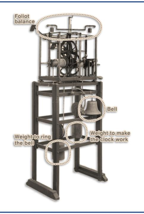
THE 1300s MARKED THE CREATION OF MECHANICAL CLOCKS THAT USED WEIGHTS TO MOVE A CLOCK'S HANDS... IN 1450, A COILED SPRING WAS INTRODUCED, MAKING CLOCKS SMALLER, AND IN 1657 CHRISTIAAN HUYGENS CREATED THE PENDULUM CLOCK THAT GREATLY INCREASED THE TIMEPIECE'S ACCURACY.
