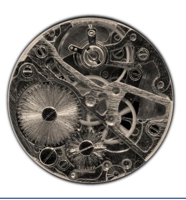
WHEN FULLY WOUND, MECHANICAL WATCHES WILL USUALLY RUN BETWEEN 24 AND 36 HOURS, AND SHOULD, THEREFORE, BE WOUND DAILY AT THE SAME TIME TO MAINTAIN ACCURACY.
